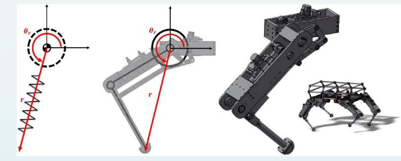
Quadrup robot leg design advanced from basic Slip model
