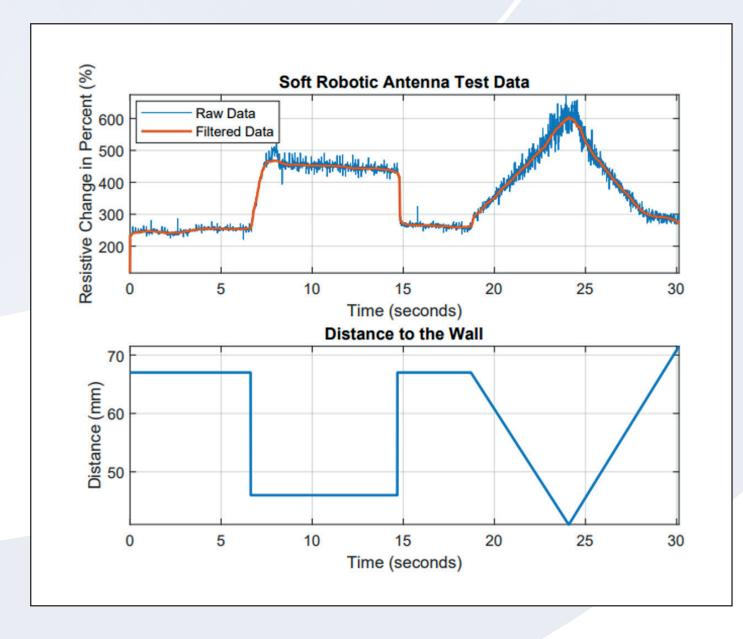
As a result of the test, a constant resistance change was observed from the moment of start, corresponding to a constant wall distance.
